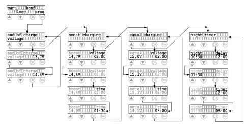
PROG). In this example, press the very rightmost key under PROG. Note that this key has the function "return to Main menu" in all other windows.
