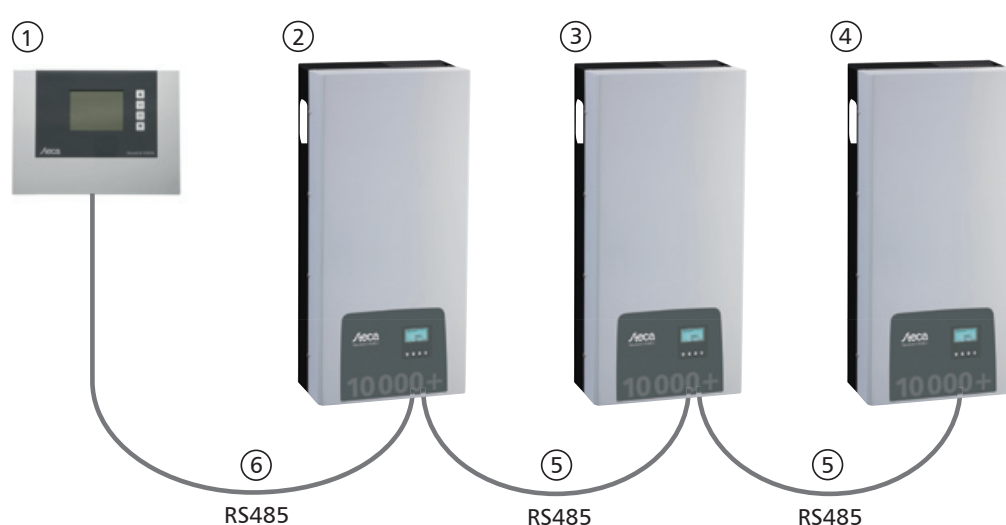
Fig. 6: Wiring diagram, using the StecaGrid Vision remote display as an illustrative example
